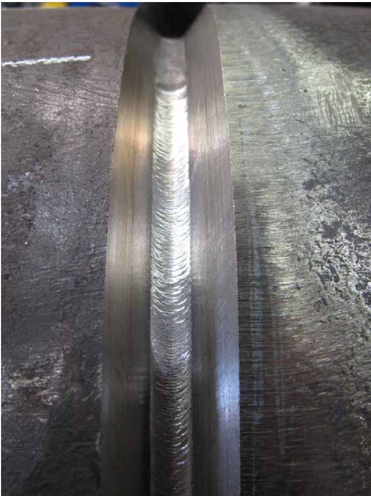
A perfectly formed GTAW root pass. With user defined seam tracking and through-arc sensing, AdaptARC can eliminate manually welded root passes for higher weld integrity.
