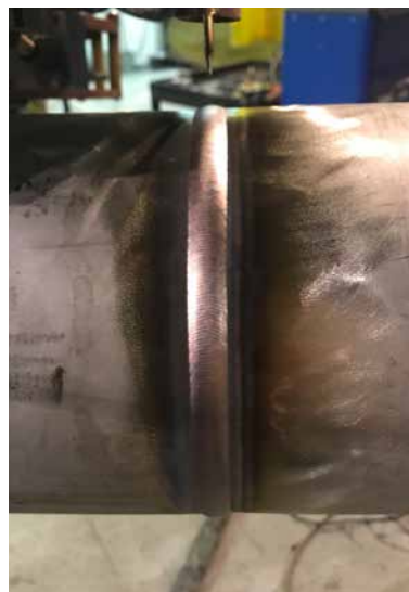
The above two photos show the outside (L) and the inside (R) of a successful open-butt automatic orbital welding procedure that was performed on Schedule 10 stainless steel.
