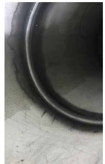
The above two photos show the outside (L) and the inside (R) of a successful open-butt automatic orbital welding procedure that was performed on Schedule 10 stainless steel.
