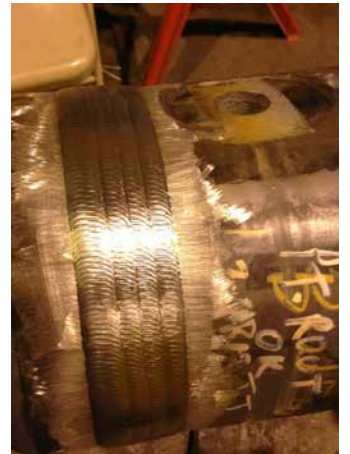
The above weld on 625 Inconel was TIG all the way out, done at an oil refinery.
